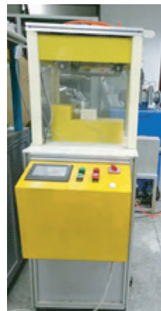
图 6 新型气泡静电纺丝设备 Fig. 6 Novel bubble electrospinning equipment
