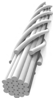
图 1 集聚区须条分层结构示意图 Fig.1 Schematic diagram of core structure of condensing zone
