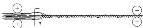
图 2 集聚区须条半自由端加捻模型示意图 Fig.2 Schematic diagram of semi-open end twisting model of condensing zone
